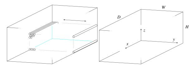
Figure 1: A container accommodating a semifluid: tubes (left); coordinate system used (right).
