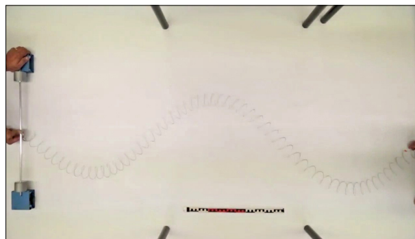
Fig. 1. Image of the spring vibration when the third harmonic was being formed. The left side of the spring is fixed while the right side is propelled manually. The calibration bar is visible at the bottom of the image.
