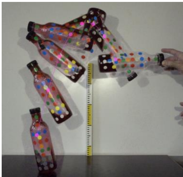
Figure 5: Stroboscopic image of the Bottle during the flip. The centre of mass is represented by pink.
