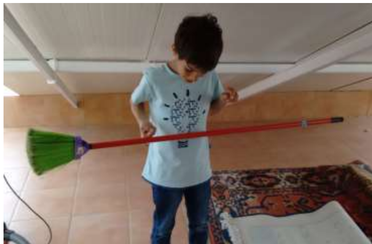
Figure 1: Estimated longitudinal position of the CG of a broom, obtained from an unstable static equilibrium technique used to find the centre of gravity. The CG is along the vertical line that crosses the wooden stick (the equilibrium is unstable because the CG is above the fulcrum).
