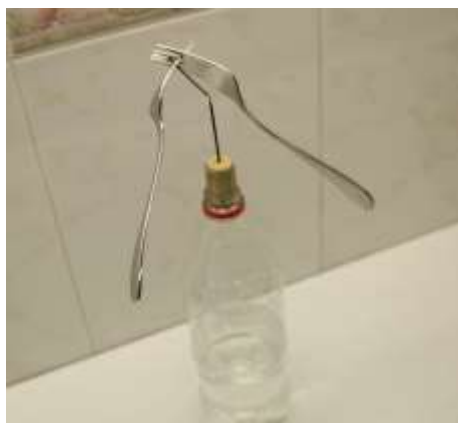
Figure 2: Estimated vertical position of the CG of the system consisting of two forks. The CG is outside the system in the intersection between the vertical gravity line that crosses the wooden stick and the forks plane, somewhere below the fulcrum.
