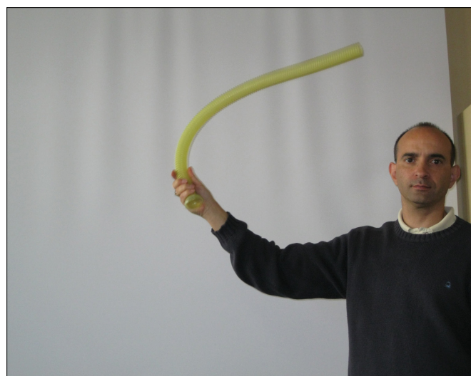
Fig. 2. Spinning of a flexible sound tube during a classroom demonstration.
