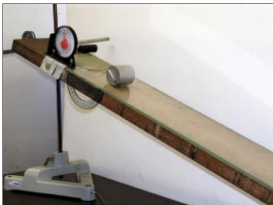
Fig. 5. Experimental setup used. The cylinder is ready to go along the incline.
