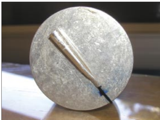
Fig. 4. One of the bases of the aluminium cylinder. The brush handle is glued in such a way that the hair stands just a bit outside the border.
