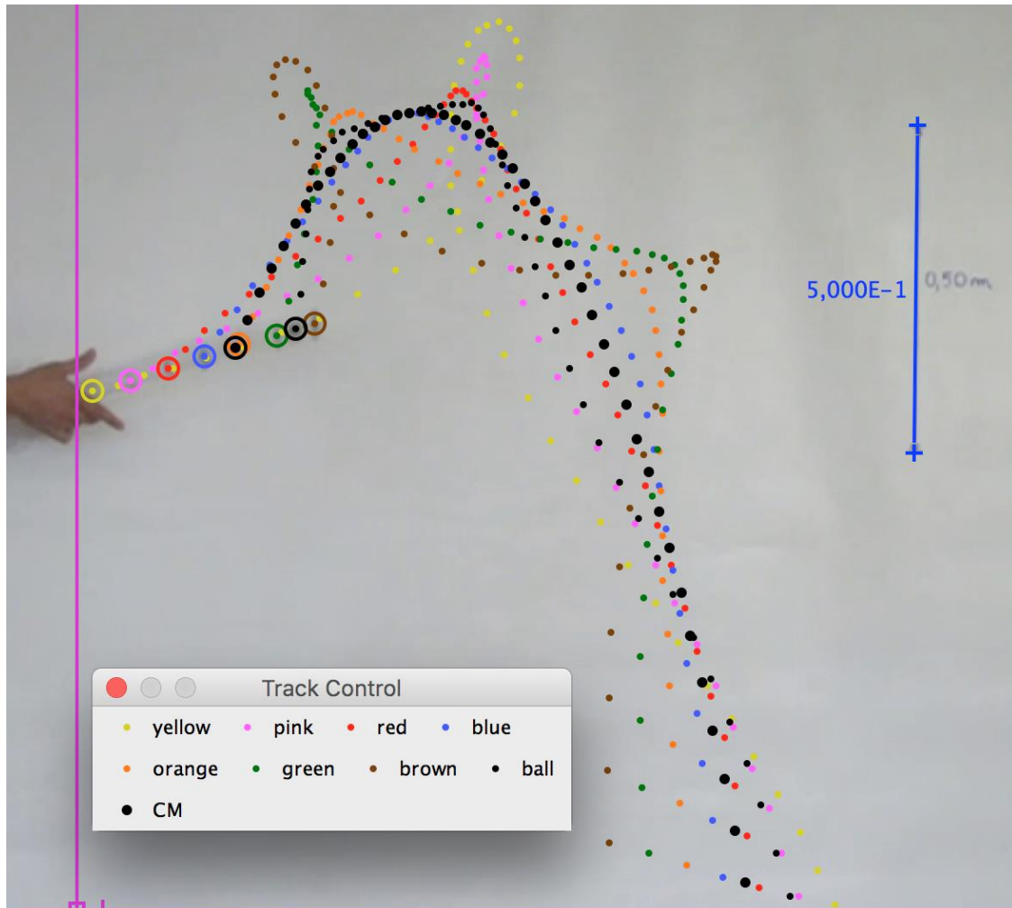
Figure 5: Trajectories of the colour markers of the body and the metallic ball. The black dots correspond to the experimental CM as computed by Tracker software using the known masses of the tube and the metallic ball, and describes a parabolic trajectory.
