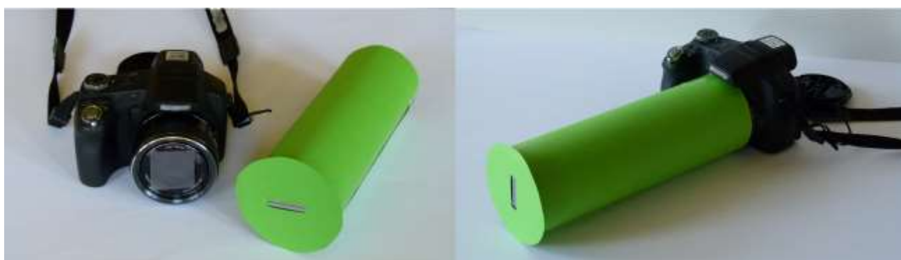
Figure 4. Photos representing the opaque tube with a slit at one end, the camera with the diffraction grating and both parts assembled. The tube guarantees that distance D remains constant for all images as well as the relative position of the slit in the images.
